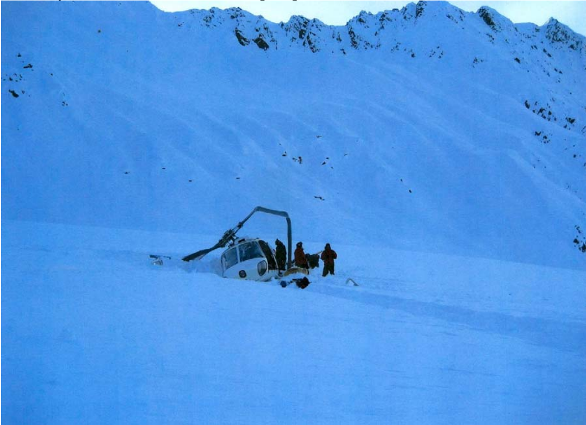
Figure 12 another rotorcraft accident involving flat light. In this case loose snow was blowing up once the rotor down wash impacted the surface. The result was a combination of flat light and whiteout conditions.
