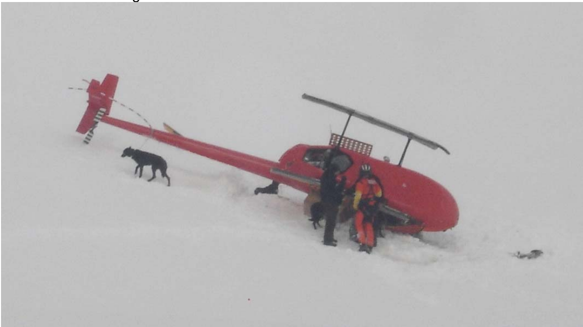
Figure 12 another rotorcraft accident involving flat light. In this case loose snow was blowing up once the rotor down wash impacted the surface. The result was a combination of flat light and whiteout conditions.
